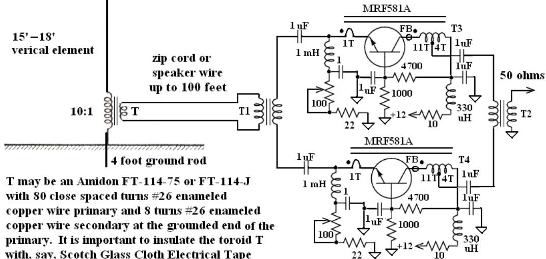
**T may be an Amidon FT-114-75 or FT-114-J with 80 close spaced turns #26 enameled copper wire primary and 8 turns #26 enameled copper wire secondary at the grounded end of the primary. It is important to insulate the toroid T with, say, Scotch Glass Cloth Electrical Tape to prevent possible shorting of turns (high permeability material is a semiconductor).**
