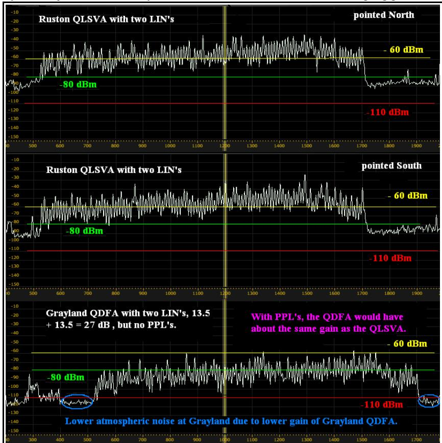
Above right are Perseus displays of the QLSVA in Ruston last night about 11 pm CDT, the 1st with maximum gain pointed due North, the 2nd pointed due South. The 3<sup>rd</sup> Perseus display at right is for the full size 100' spaced Grayland QDFA about midnight PST two years ago. It is seen that the QLSVA has about 30 dBi more gain than the full size 100' spaced standard QDFA (without supercharged PPL's). This is about 20 dBi more than EZNEC calculated. Measurements have shown that
