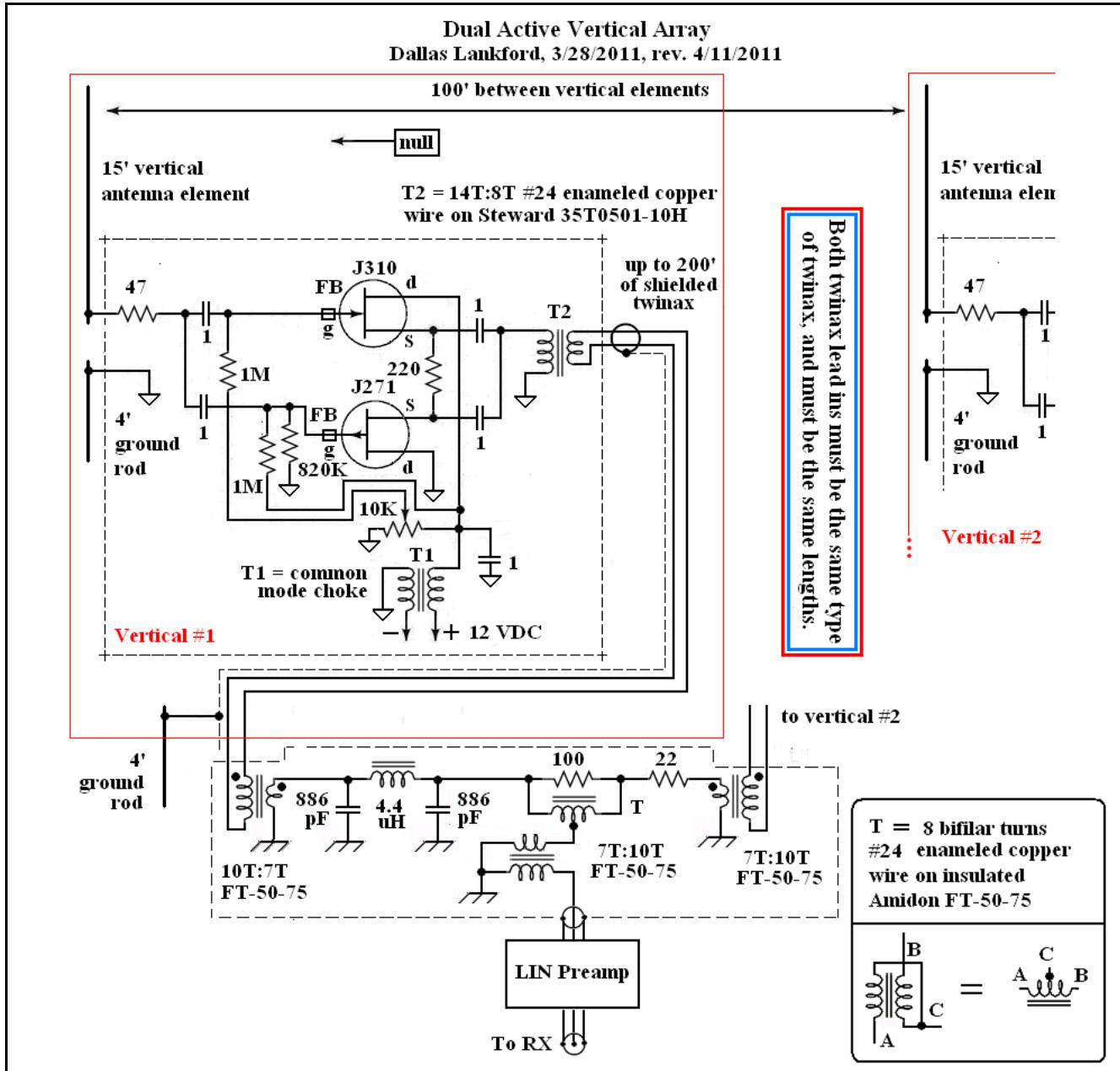
The tests initially had about the same outcome as two years before with passive verticals, namely poor or nonexistent nulls for most MW frequencies. In the meanwhile I had read about vertical arrays with negative real parts of some of the source impedances, how they were caused by mutual antenna impedance, and how they led to phasing and other problems. The solutions I read about involved resonating the vertical arrays, which did not appeal to me because I wanted broadband
